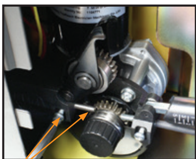
(10) Loosen the inlet guide tube retaining screw.
