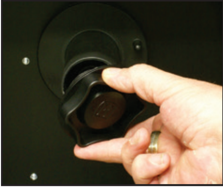
(1) Remove the spool retaining nut.
